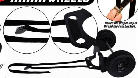
1. Weave the long strap through the holes in the wheel bracket in this pattern, avoiding twists, with the cam buckle facing down. Do not thread the cam buckle vet.
