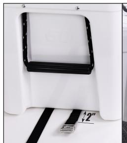
**2** Drop the cooler down onto the wheel bracket (drain plug side) with the long strap stretched out under the cooler in the pattern from step 1. Keeping the strap free of slack, make back up thru the cam buckle, but do sure the cam buckle is positioned no more than 2 inches from the cooler.
